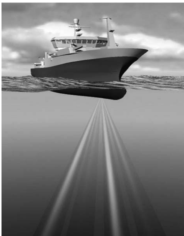
Fig. 5.27 The Acoustic Doppler Current Profiler (ADCP) as a shipboard installation. Four beams are projected, each about 30^\circ off the vertical, giving radial velocity components from the echoes at each depth. (Redrawn from Demer et al. 2000.)
